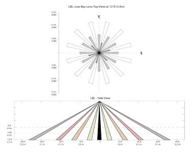
Note: The application/absolute range of the sensor is subject to variation because of different types of clothing, backgrounds, and ambient temperature. Therefore, ensure that the lens is properly oriented along routes with expected traffic and conduct testing along those routes.
